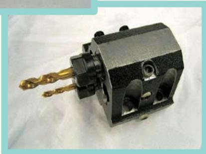
The center alignment drill holder photographed below adopts an eccentrically structured drill insertion part and shank. The holder is compact enough to fit in a two-hole holder.
