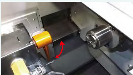
Wavy Nozzle installed inside a TAKAMAZ XG-4. It is compact and takes up little space. The nozzle swings in the directions indicated by the arrows.
