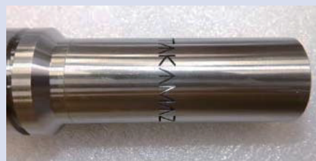
Profile cutting of “TAKAMAZ” by piercing
