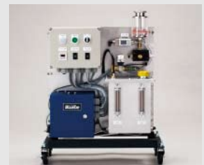
Generates and sprays mist of water-soluble coolant.
