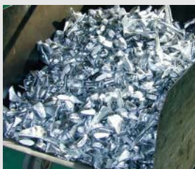
In the aluminum piston casting factory, chips and scraps can be put into the re-melting equipment without drying them.
