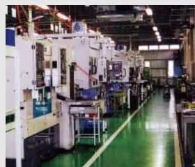
Clean shop floor without oil spills thanks to semi-dry cutting. Shop floor soling is significantly reduced and workability is improved.
