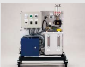
Coolant mist equipment Sprays mist of water-soluble coolant
