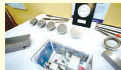
Staging exhibits with the focus on craftsmanship to create highly accurate flat surfaces (scraping)
