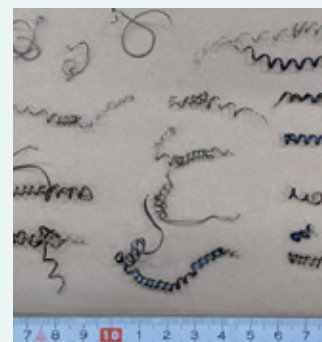
Chip breaking movement applied
