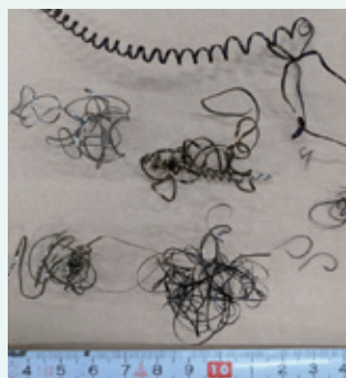
No chip breaking movement
