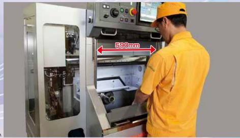
A full-width door above the holder mounting position. The door opening is 590 mm wide.
