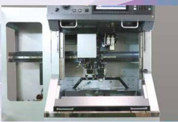
The "WA30" compact servo loader utilizing upper space in the machine is adopted to meet the user's needs.
