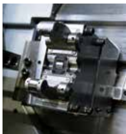
Steady rest that proves effective with long workpieces (Made by SMW, Model: SLU-X-1)
