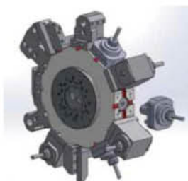
BMT55 Maximum tool size: \phi 20 mm
