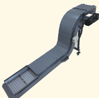
● Chip Conveyor (Floor type) The system where linked steel plates are moved to transport chips has the advantage of efficient transport regardless of the material or status of the chips.
