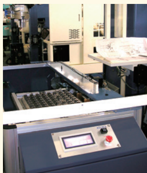
● Tray Changer Workpieces can be stored in individual trays.
