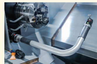
● Tool presetter Adjusts the position of the tool tip to substantially shorten setup times. In-machine (touch sensor method) and external types are available.
