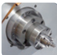
【Chuck】 (Left) OP-1 : KITAGAWA N-06 (3-jaw) (Right) OP-2 : TAKAMAZ TIC1-N3
